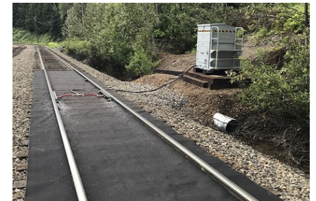
Flange grease is applied to the gauge face of the rail before entering curve
