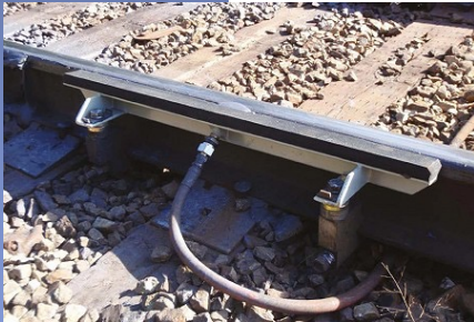
TOR Friction Modifier is applied on top of rail
