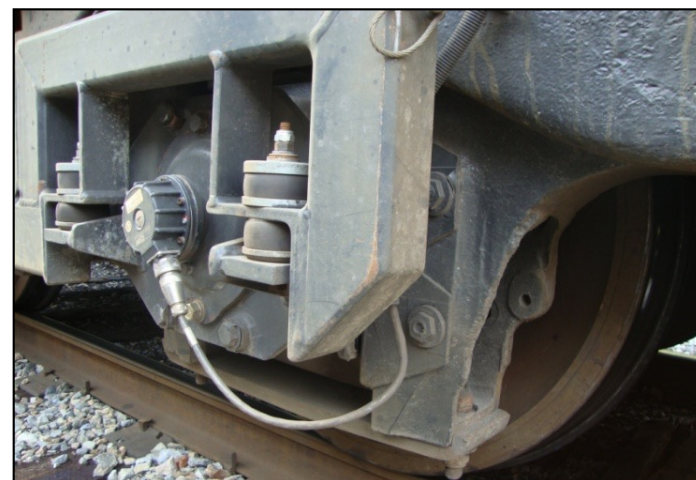
Encoder on the left rail of the lead truck middle axle
